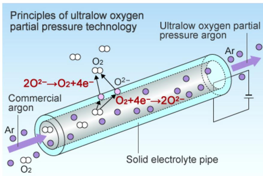
It is well known that ions can move in liquid, like the electrolytes in rechargeable batteries. Some solid materials have same property. Materials with this characteristic are collectively known as solid electrolytes.
